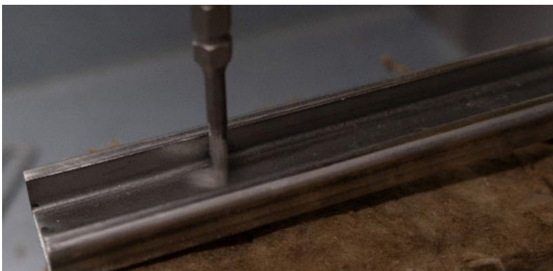
Figure11 – Drilling of pilot hole
