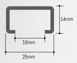
The 25/14 channel is available in 2700mm lengths and features closely spaced pre-punched holes to ensure a fixing position is always near the end, even when cut on-site. The channel has a 16mm opening to easily accommodate washers and fixings.
