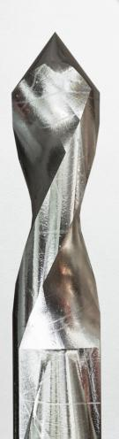
SuperTEK® 7 double-helical point consistently provides industry-leading drilling performance due to its aggressive rake and flank angling and honed blade-edge. This product will self-drill and self-tap in mild steels from 4.0 mm to 18.0 mm in overall thickness.
