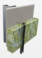
2. INSTALL FIXING THROUGH CHANNEL AND SLEEVE BACK TO INTERNAL STRUCTURE.
