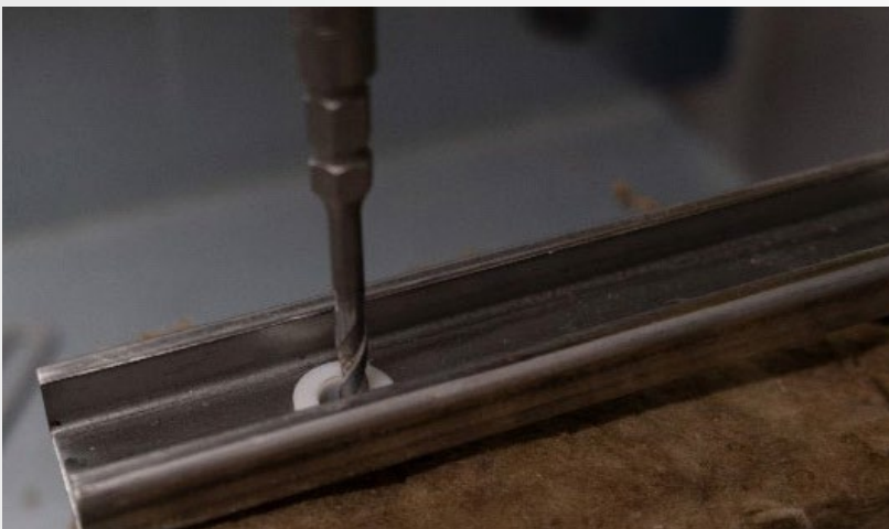
Figure11 – Drilling of pilot hole
