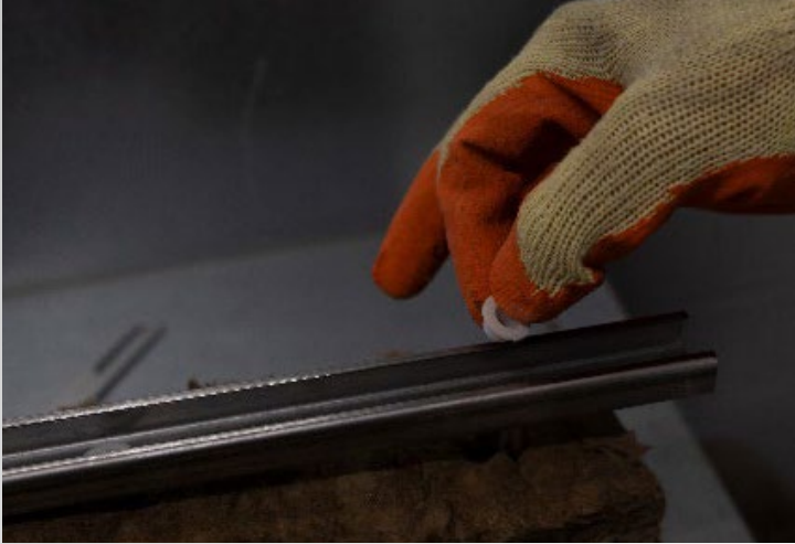
Figure 09 – Seating of nylon shoulder washers
